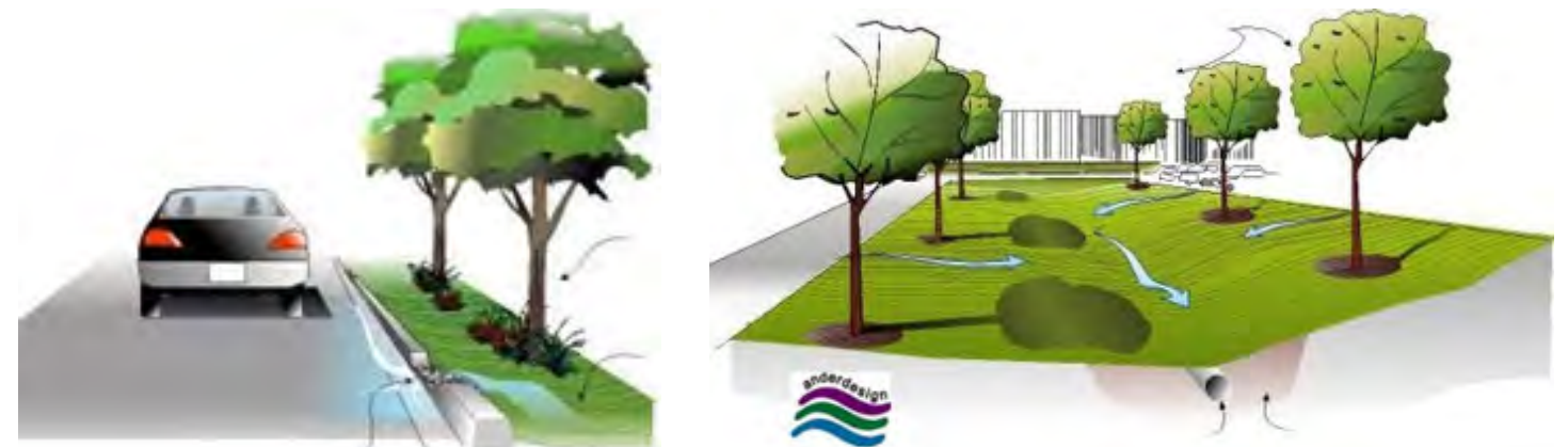
Sustainable stormwater design, directing runoff into vegetated parkway to absorb and filter water.
