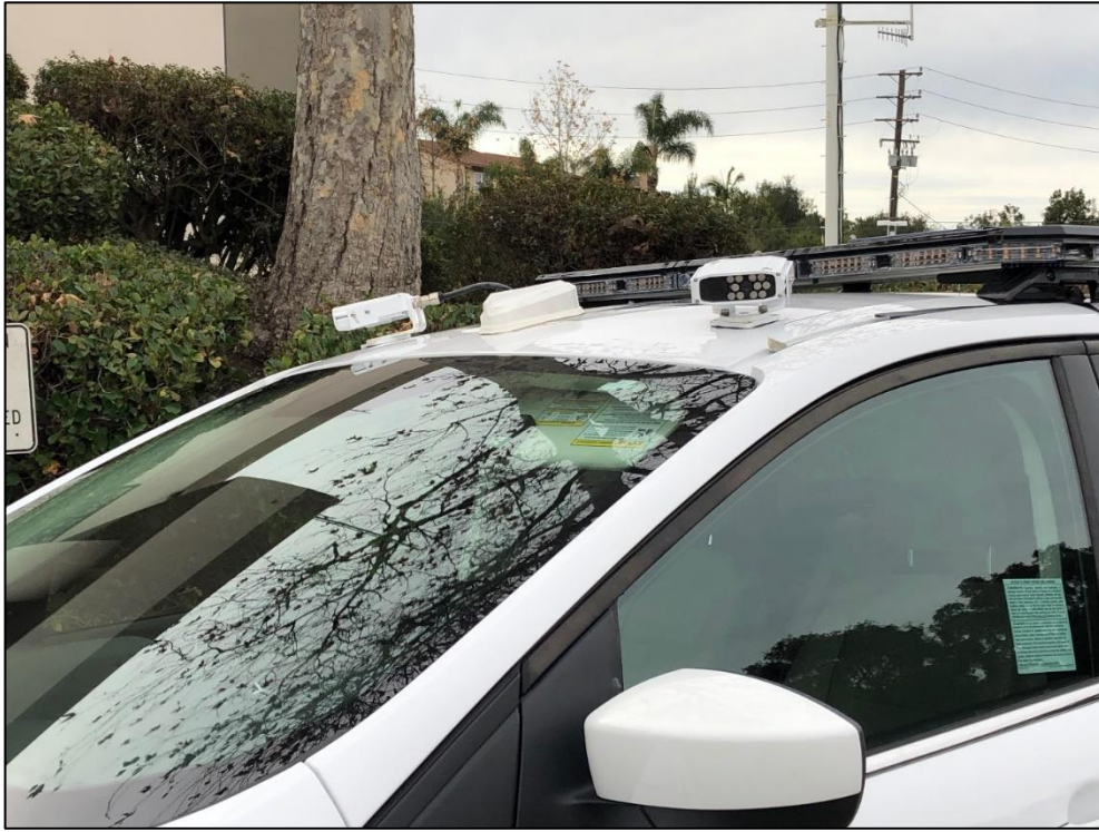
Image 6. LPR Mounted on City of Seal Beach Enforcement Vehicle
