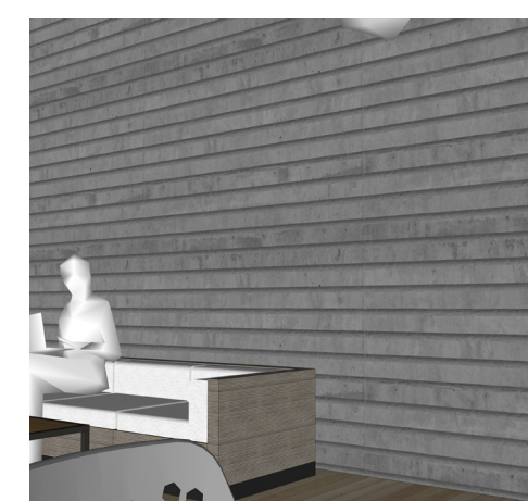
16. BOARD FORM CONCRETE PLANKS
