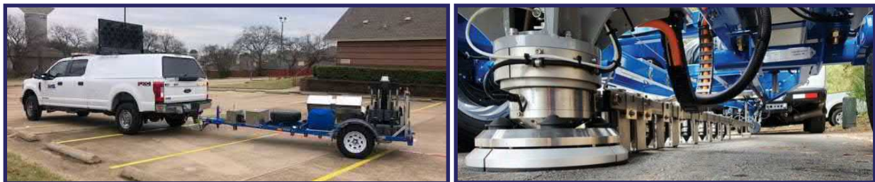
Figure 10 - Fast Falling Weight Deflectometer
