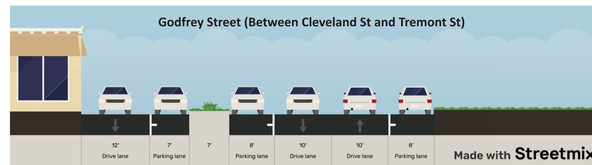
Cross-Section A-A: Existing Conditions
