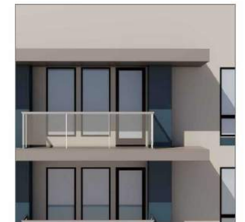
EXTENDED FLOORPLATE AT BALCONY
